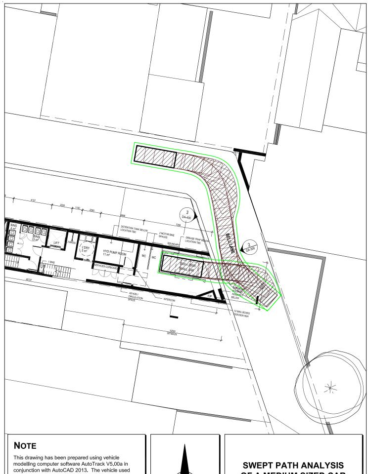
This drawing has been prepared using vehicle modelling computer software AutoTrack V5.00a in conjunction with AutoCAD 2013. The vehicle used is based upon vehicle data provided by Austroads and incorporates a reasonable degree of tolerance. However, it is not possible to account for all vehicle types/characteristics and/or driver ability.
